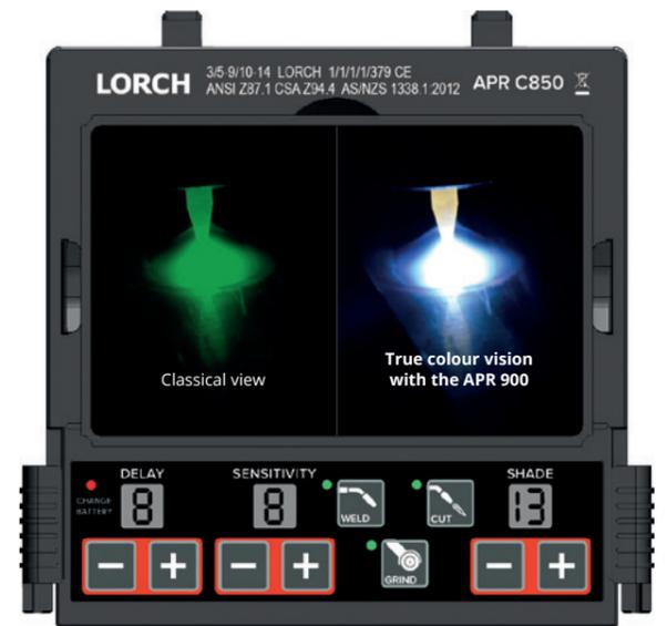
**Operation and operating modes:** Option of setting operating modes, protection level, delay, and sensitivity with clearly marked buttons and a display that can be read at any time. Welding mode (protection levels 10-14), grinding mode (protection level 3), and cutting mode (protection levels 5-9) are available for selection during operation.
